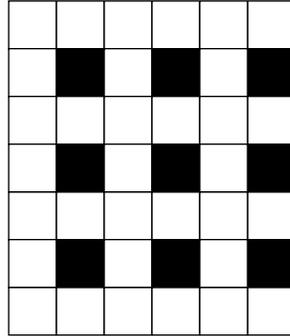
where a black square represents a hole. No conductor will be defined in that square region. Further local discretization can be accomplished with other `contact` utilities as described earlier in this section however there is no utility for discretizing more finely around every hole.
