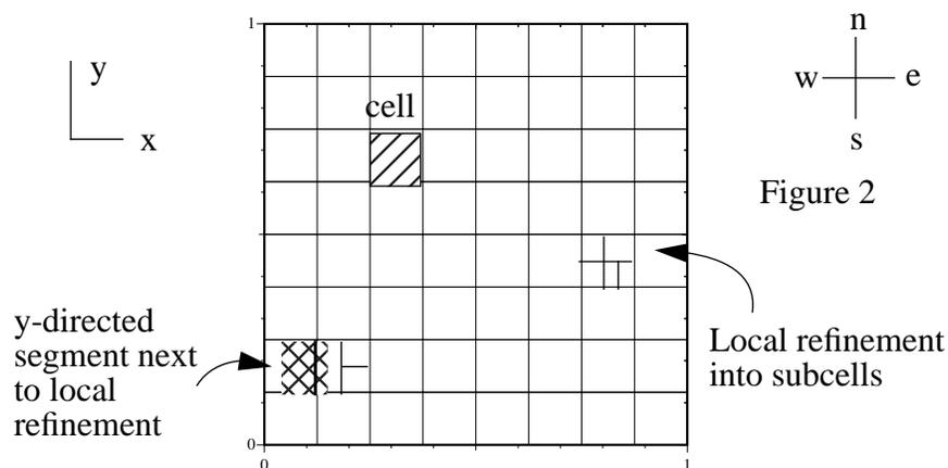
To accomplish local refinement, a cell can be divided into subcells. After refinement, all line segments will correspond to a segment of conductor whose current direction is along the length of
