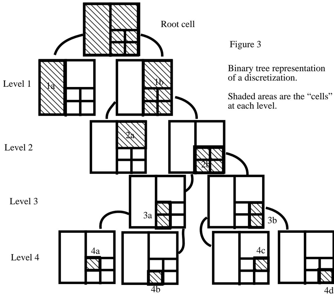
that at the top of Figure 3, the entire plane is represented by one single cell as shown by the root cell in the figure. It's two children are formed by dividing it into two east-west portions. The west portion, shown as the left child, is not discretized further and is a leaf cell in the tree at level 1. At level 2, there are two cells resulting from the north-south division of the east cell at level 1. The north cell is a leaf cell since it is not further discretized.
