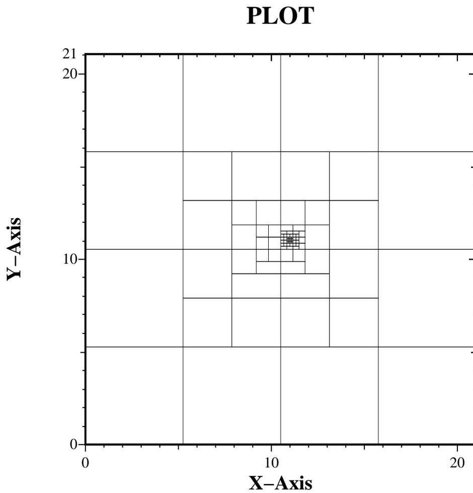
Note that the  $x_c/x_r = 0.1/0.2 = 0.5$ . Choosing this ratio closer to 0 produces more gradual refinement. The opposite is true for the ratio closer to 1.
