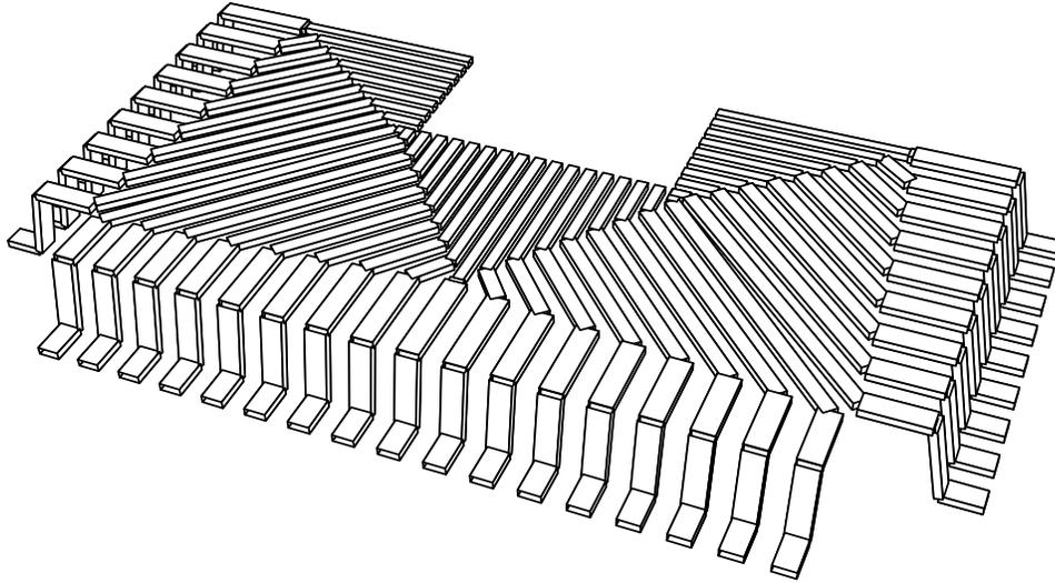
Figure 8: Thirty-Five Pins of a 68 pin Cerquad Package
